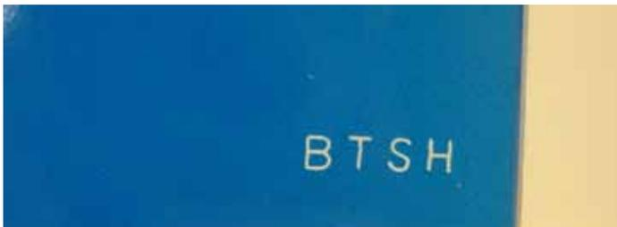
“Our packaging is chipboard material, so we are typically removing the outer, colored layer and exposing the white substrate underneath,” he says. “The characters are well-defined and provide a nice, crisp look.”
